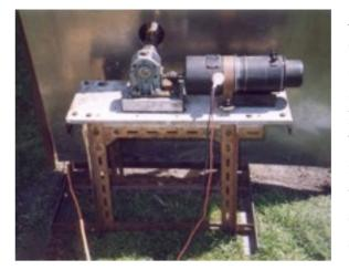
As the motor may have to work continuously for nine hours or so, anything which eases the load is to your advantage. You may even work a simple hand cranked alternative using Dexion brackets for example in the event of the motor failing. Since the aim is to cook the meat evenly, a rotation of 40 degrees every ten minutes might be as effective as a continuous rotation.
